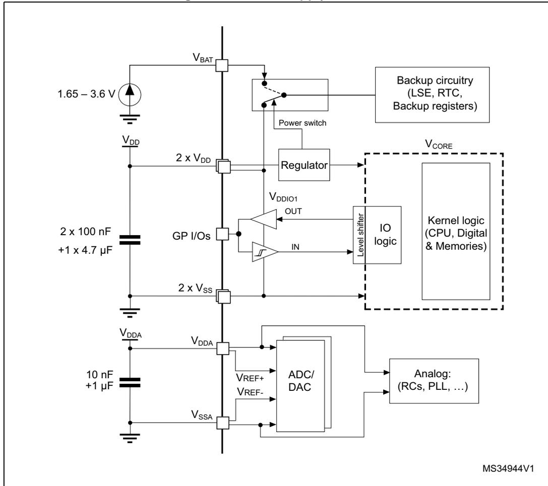
**Caution:** Each power supply pair (V<sub>DD</sub>/V<sub>SS</sub>, V<sub>DDA</sub>/V<sub>SSA</sub> etc.) must be decoupled with filtering ceramic capacitors as shown above. These capacitors must be placed as close as possible to, or below, the appropriate pins on the underside of the PCB to ensure the good functionality of the device.
